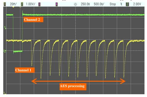
A power consumption waveform like the one in the above picture is expected.
